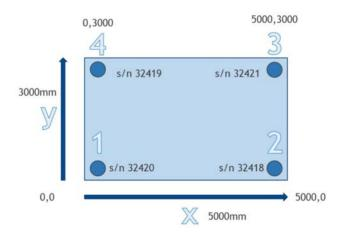
Now you will get read-outs of the load placed on each load cell, total weight, as well as a display of the center of gravity. The larger the circle the larger the weight.
