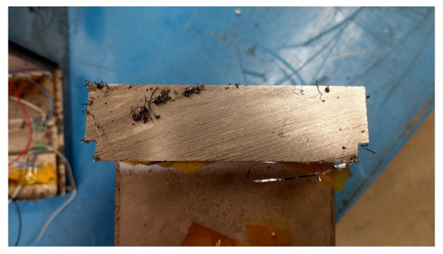
Top down close up shot of the side that snapped in the destruction test
