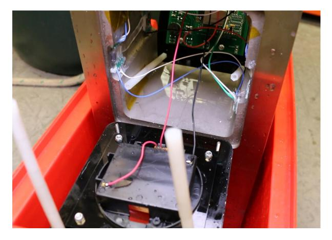
When the batteries were reconnected the display panel initially turned on, performed general booting sequence and then shut off. Nothing showed on the screen and the unit failed to function when force was applied to it in order for it to display a measurement.
