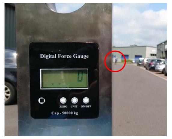
Figure B – Showing test setup with handheld being walked away from load cell by tester
