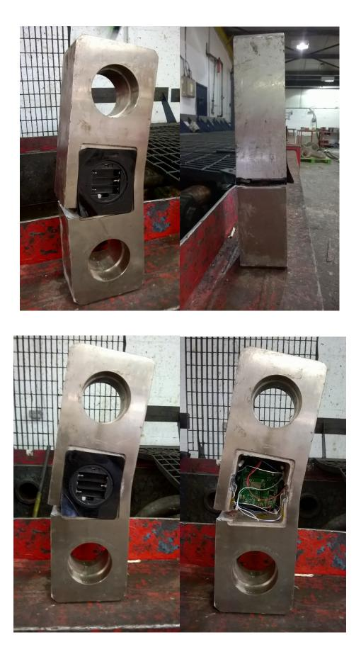
Photos of the load cell after it has yielded in the destruction test. As you can see it has snapped only on one side, which is highly unusual:
