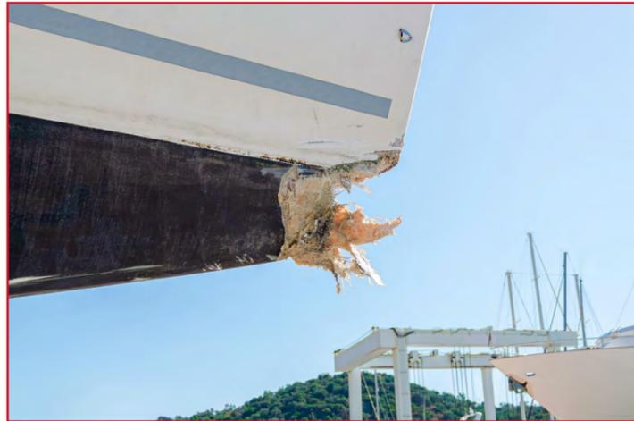
Damage to a ship after a bollard overload failure
