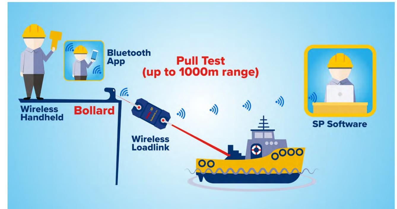
Bollard load testing and bollard pull testing for tugboats
