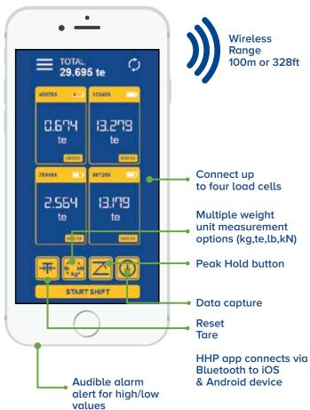
Designed to replace outdated mechanical products still in the field, this 14,300lb (6500kg) Dynamometer, the 'BlueLink', is the latest SP product to feature their proprietary Bluetooth wireless technology.
