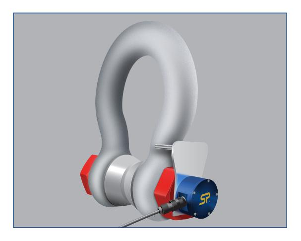
Available from stock in capacities 3.25t to 120t, and available up to 1,550t, the Loadshackle is manufactured from Crosby's industry leading 2130 Carbon and 2140 Alloy Bolt Type Anchor Shackles (3.25te - 120te) and the GN H10 Alloy Bolt Type Anchor Shackle (120te on up). The Loadshackle offers reduced overall weight and headroom providing a great fit for low headroom applications.
