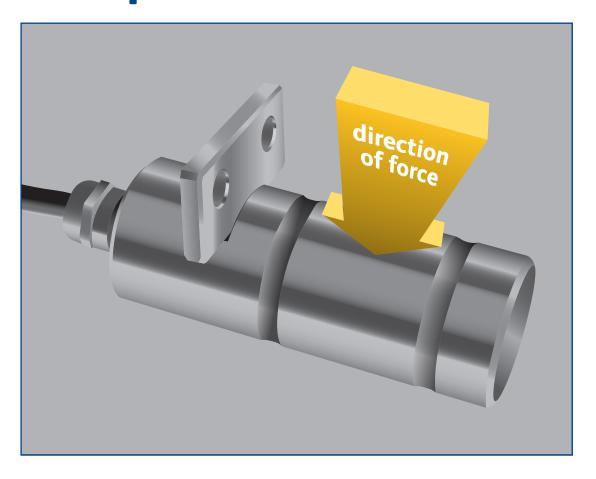
The Straightpoint range of Load Measurement Pins are designed for general use. They are machined from high tensile stainless steel and are normally supplied complete with an anti-rotation plate.
